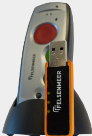
You can configure the SHALOSH ECO using the SERVICE-STICK. Just place a SIM card into the SHALOSH ECO, put it into the charger, wait until it announces itself to the SERVICE-STICK and then configure it. This is faster than a configuration via SMS, especially when many parameters have to be configured.
